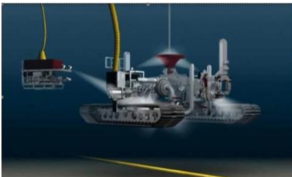
Figure 5.1 Subsea 7 i-Trencher proposed for use during pipeline installation operations
